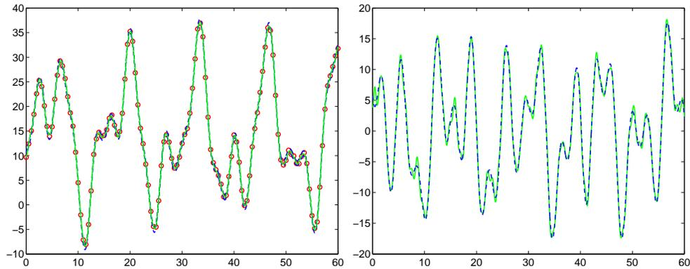
FIG. 7.2. Left: The functions  $h + 0.5$  and  $h - 0.5$  from Example 7.2 are shown as blue dashed lines. The perturbed sampling points  $(k/2, h(k/2) + e_k)$  with  $e_k \in [-0.5, 0.5]$  ( $k = 0, \dots, 120$ ) are the centers of the red circles. The reconstructed function  $\tilde{h}$  is shown as a green line. Right: The function  $h'$  from Example 7.2 is shown as a blue dashed line. The derivative  $h'$  of the reconstructed function is shown as a green line.
