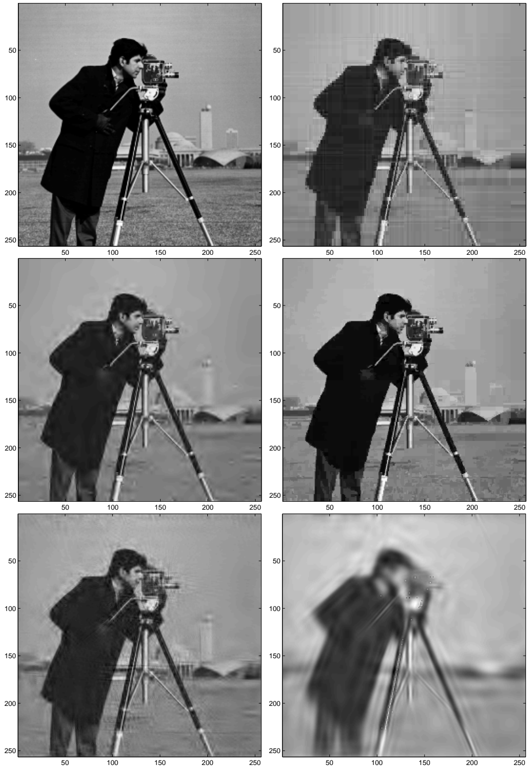
Figure 8: Approximation of the 'cameraman' image with 2048 coefficients. See PSNR values in Table 2. (a) Input, (b) classical Haar, (c) Biorthogonal 9-7, (d) Tetrolets, (e) Contourlets, (f) Curvelets.
