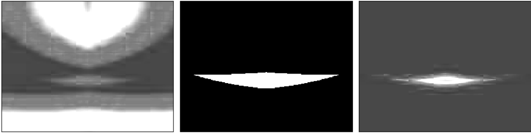
Fig. 9.22: Estimation of the center point C as the maximum of R(C')I(C') (right) where R is a distance function (left) and I is a probability function (middle).
