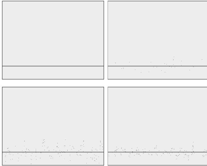
Fig. 9.9: Reconstructed back wall cluster for different noise levels.
