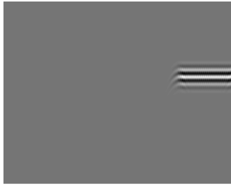
Fig. 4.13: Modelled ToFD output data for a crack defect.
