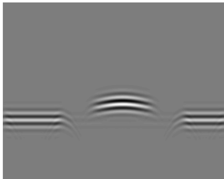
Fig. 4.15: Modelled back wall thickness measurement.
