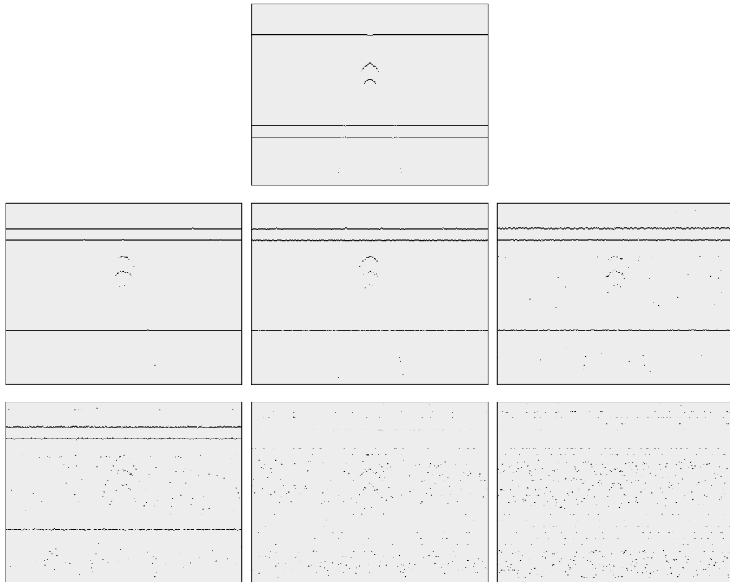
Fig. 9.20: Non-zero elements of deconvolved data for different noise levels, special weights were used for the two highest noise levels (bottom, middle and right).
