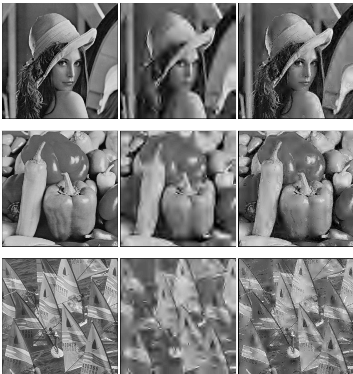
Figure 4: (Left) Original image; (middle) tensor product wavelet transform with 9/7 filter, keeping only 500 nonzero coefficients (nzc); (right) our hybrid method with 9/7 filter, keeping only 500 nzc.
