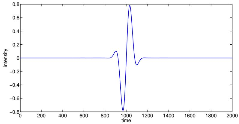
Figure 16: The pulse function used by the ultra sonic scanning devise for non destructive material examination.
